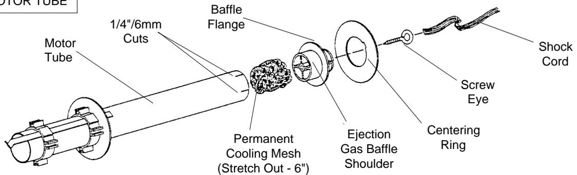
1. Make four 1/4" (6mm) long cuts, 90 degrees apart, in the front end of the motor tube.
