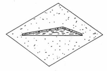
Cut and lightly sand the balsa fins with fine sandpaper.
