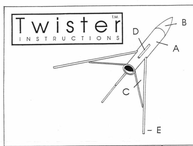
Body tube (ET-20) Α (BC-20) В Nose cone (BAL10007) C Balsa (LUG125) Launch lug D (Dowel10007) Ε Dowel (3) F Decal\* (D10007) (TEM10007) Template\* G \*Items not shown
