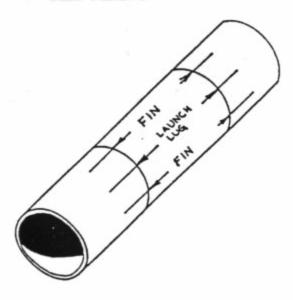
Cut out the fin marking guide and wrap it around the body tube. Mark the fin and launch lug locations with a pencil.
