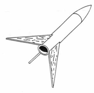
Glue the three fins to the fin location marks, one at a time, with white glue, to the body tube. Wait for all the fins to dry throughly.
