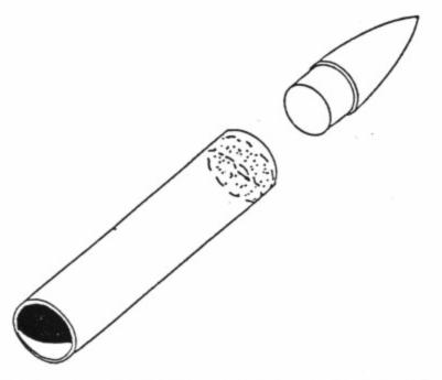
Apply white glue inside the end of the body tube. Insert the nose cone so it touches the glue and put aside to dry.
