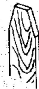
B. SAND TAPERED PORTION TO SHAPE
