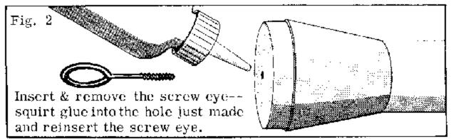
STEP 5. Assemble the parachute according to the instructions in the kit. Prepare a shock cord anchor as shown and install the unit inside the main body tube 1/2" from the forward end.
